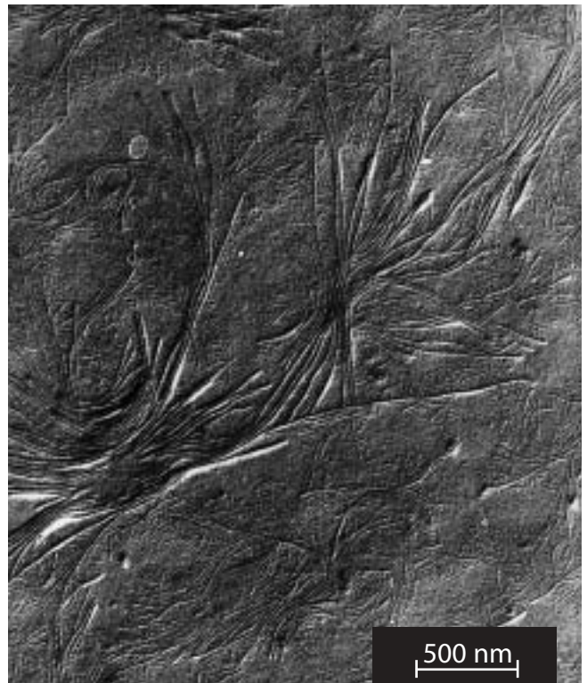
Figure 3: Photo of a polytetrahydrofuran-rich PA 12 elastomer taken under a transmission electron microscope.
